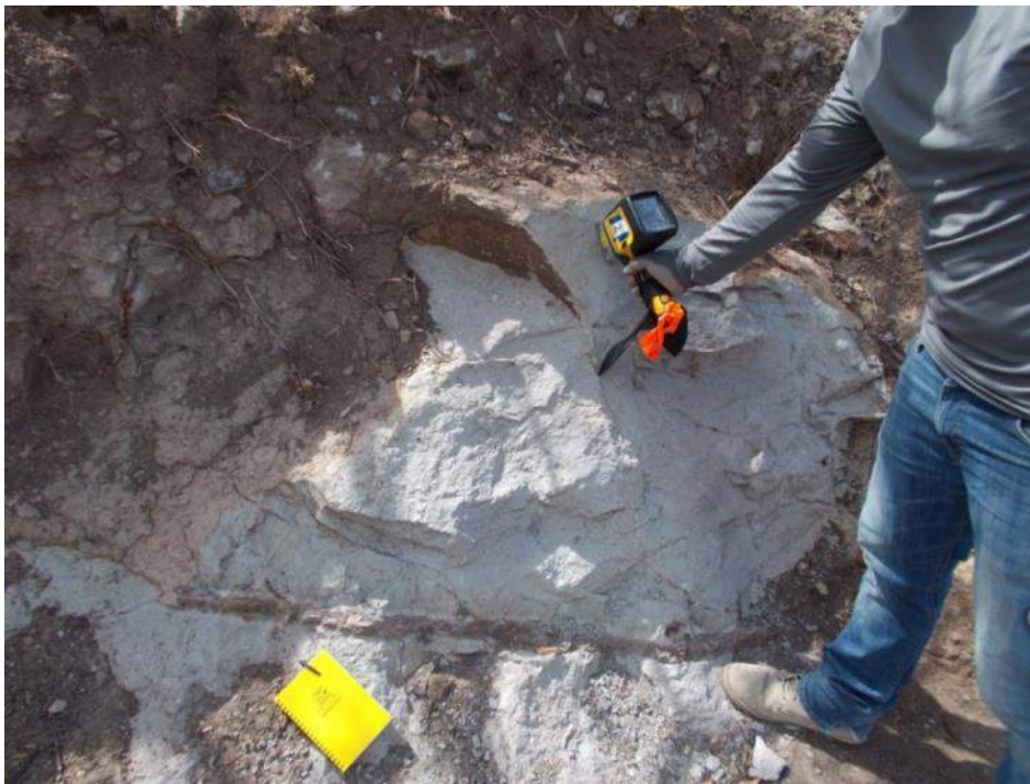
Photo 2-2 Outcrop of tuff with 197 ppm silver by pXRF
